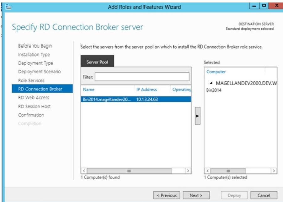
Figure 8: RD Connection Broker/Add Server Name
